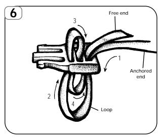
**To tighten waist belt,** feed the anchored end of the waist belt up through the buckle to form a loop. Pull the free end of the waist belt through.
