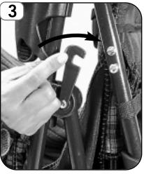
Lower the clip located on the side of the stroller frame.
