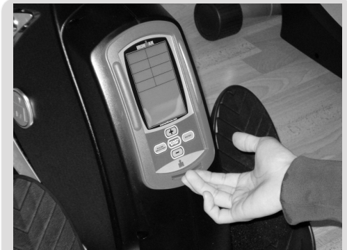
The miles / kilometer switch is located on the back of the console. To remove the console, push in the tab of the lower part of the console and lift up.
