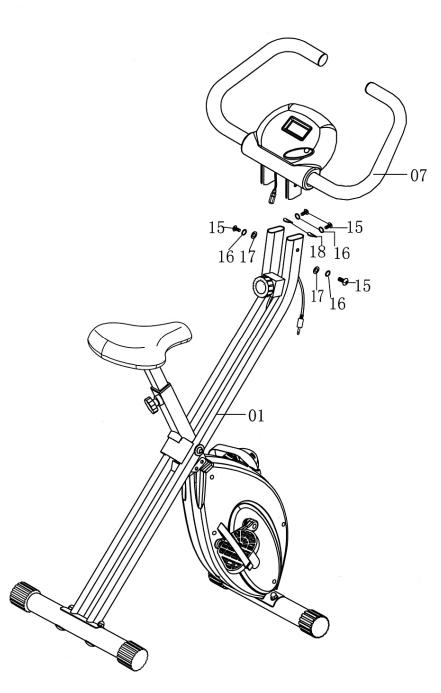
STEP 6 (See Diagram 6) A.) Connect Sensor Wire (#20) from the front post of the Main Frame and connect to the Computer wire (#19) from Computer.
