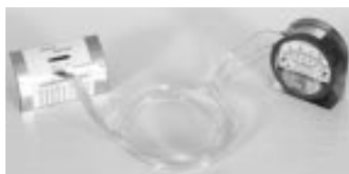
figure 11.6 Magnehelic Gauge with Air Flow Grid
