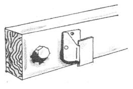
Before hanging the dryer on the wall please note that the plastic spacer should be located as illustrated.
