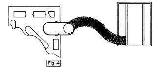
Replace the existing exhaust air director on the back of dryer with the adapter. Mount vent kit in sideways or upward position on the back of dryer using the same fasteners (Fig.-4). Direct other end of hose outside the window.
