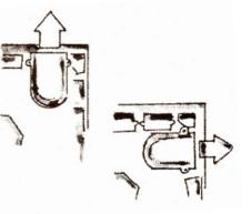
Note: The exhaust air deflector on the back of the dryer can be positioned as shown to exhaust upward or sideways.
