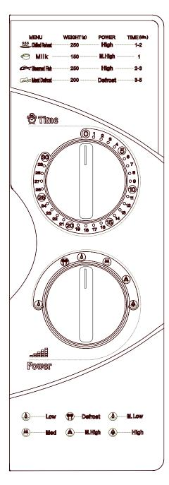
The control panel consists of two function operators. One is a timer knob, and another a power knob.
