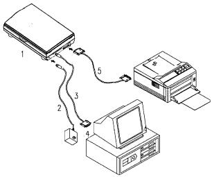
Figure 2-2 ImageReader ScanPro scanner cable connection
