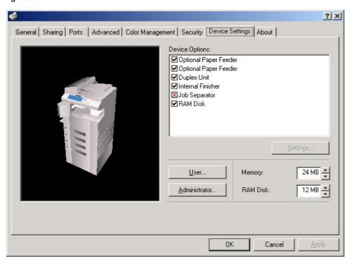
To access the Device Settings screen, in step 4 on page 2-1 select [Properties] from the menu and then click on the Device Settings Tab. When you have added optional equipment, make the appropriate settings for that equipment here. Once the corresponding setting is complete, the corresponding function of the installed option will be added to the printer.
