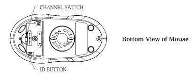
Step 7: Use the slide switch in the battery compartment of the **mouse** to select the same channel as the one selected in step 2 and 5. (Open the battery compartment cover to find the switch channel setting)
