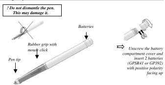
⇒ Slide an ink refill into the pen tip (standard M21 refill of 67.0mm long X 2.35mm) and press it gently until it is correctly lodged.
