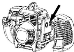
The muffler is designed to reduce the noise level and to direct the exhaust gases away from the operator. The exhaust gases are hot and can contain sparks, which may cause fire if directed against dry and combustible material.
