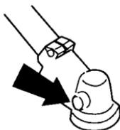
The grease in the bevel gear does not normally need to be changed except if repairs are carried out.
