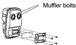
**CAUTION!** Never use a machine that has a faulty or loose muffler. Ensure the muffler bolts are tight.
