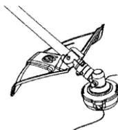
**WARNING!** Never use a cutting attachment without an approved guard. See the section on “Technical data”. If an incorrect or faulty guard is fitted this can cause serious personal injury.
