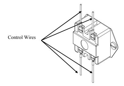
4. Remove the two (2) mounting screws or disconnect from thermostat, as required.
