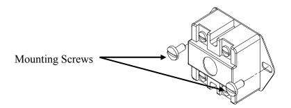
5. Replace control and install new high limit switch by performing above steps in reverse order.
