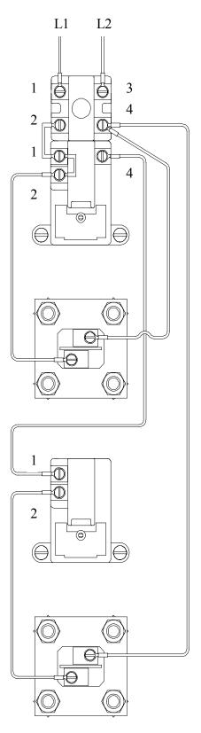
Interlocked for Non-Simultaneous Operation
