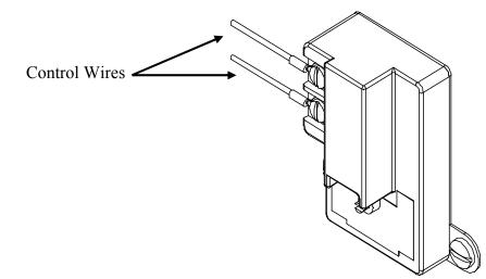
4. Remove two (2) mounting screws and disconnect from high limit cut-off, if required.
