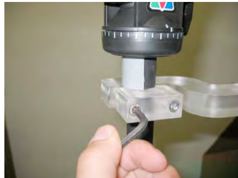
Fig 3- Attach vertical Assembly- Ensure the Vertical Actuator Rod will have adequate clearance and will not hit the tripod leg.
