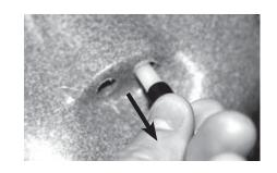
7. With the old tubes and lines removed, install the new tubes with lines that are in this kit into the holes that you just removed the old tubes from. Getting the end fittings into the holes will be a tight squeeze, so you may need a small hammer to tap them into the holes so that they are fully installed. *IMPORTANT: When these lines are installed, the right line will be for the DOWN control and the left line will be for the UP control.*
