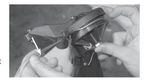
Thread in the bolt to hold the two halves together. IMPORTANT NOTE: DO NOT SCREW DOWN THE BOLT SO THAT IT IS TIGHT. YOU ACTUALLY WANT IT TO BE A FAIRLY LOOSE CONNECTION ALLOWING AN 1/8"-1/4" OF MOVEMENT. IF IT IS TOO TIGHT, THE RUDDER WILL NOT GO UP PROPERLY.
