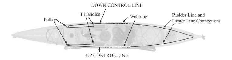
29. Your up/ down rudder system is now ready to go a. Pull on the right "T" handle to lower the rudder. Pull the line tight and cleat off to hold it in the down position. b. To raise the rudder, uncleat the lock down line and pull the "T" handle on the left side of the boat. IMPORTANT! When the rudder is in the locked down position, it will have some flexibility in the system due to stretch in the rope, but it should be uncleated and raised prior to beaching.
