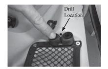
16. Drill a hole in the dotted location with a 5/16" drill bit
