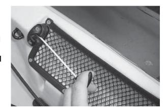
30. Place the stickers on the "T" handles to label which one does what. The "UP" sticker should go on the left handle and the "DOWN" sticker should go on the right handle. To ensure a good adhesion, make sure that the handles are clean of any water or debris.
