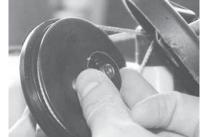
As you insert the rudder half into the housing, you have to be careful to not allow the rudder lines fall off the track around the circular rudder drum. To prevent this, pull up on the up/down control lines that are exposed on the deck to remove the slack and keep the lines tight around the drum.
