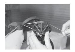
12. Slide the bolt through the rudder portion of the assembly and place the plastic washer over the threaded end. Insert then end of the bolt into the housing and bolt the rudder assembly back together.
