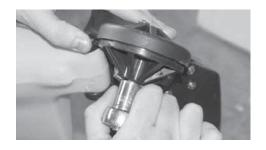
13. Take the ends of the lines that you fed through the rudder and make the loop so that it is small enough to pass a screw head through. The size of the loop isn't that critical, but do not make it any more that 3/4" big. See the pictures below on how to tie the knot needed for this loop
