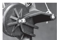
5. Pull on the lines that exit the hull so that they completely pull out of the rudder housing.
