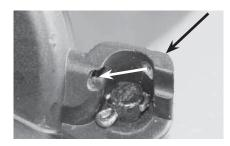
10. Feed the DOWN control line into the upper hole on the rudder part of the assembly and tie a knot in the end of the line to keep it from pulling through.
