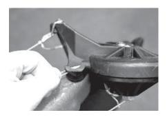
6. With the up and down control lines loose, pull on them and remove them from the hull with the tubes. If they get hung up inside the hull, you can cut whatever is preventing you from taking out the lines. You will no longer need these lines and tubes with this kit.
