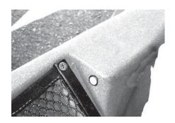
21. Remove the nuts that bolts on the block that routes the mainsheet back to the forward deck mounted bar. The screws themselves don't need to be removed, so just take off the nuts.
