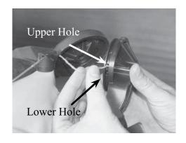
11. Now feed the UP control line through the same two holes above the rudder pin to the inside of the rudder housing. Wrap the line so that it goes over top and around the drum. Insert the end of the line into the lower hole indicated in step 10 and tie a knot at the end of the line.
