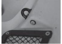
18. Locate the cleat on the right side map pocket just like in step 7 and use the holes in the cleat as a guide to drill two 11/64" holes through the map pocket frame and kayak hull material underneath it. Make sure to center the cleat along the width of the map pocket frame so that it rests on a nice flat surface.
