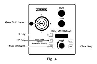
At Idle, the timer display [--:-] shows that no time has been set (Fig. 4).
