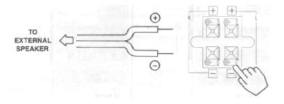
**CAUTION:** Do not connect Speakers simultaneously to the REAR SPEAKER terminal of the Projection TV and Amplifier. This could damage both the Projection TV and the Speakers. Your Hitachi TV was designed to use 8 speakers only. Any other type may degrade the audio performance of your entertainment system.
