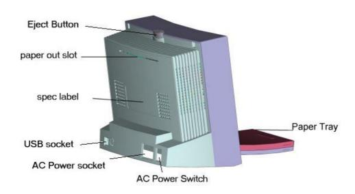
2. Connect "USB Cable" to printer. Connect the other side to PC.
