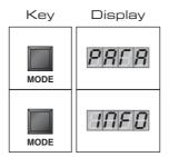
Press "STEP" until the system displays the information you need. The point located behind the first position flashes to indicate that the boiler is in "INFO" mode.
