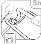
Stand behind the mower and hold the handlebar with your left hand. With your right hand hold the engine start - grip and pull slowly until resistance is felt, then pull rapidly to crank the engine. Carefully return the start grip to the storage position when the engine starts.
