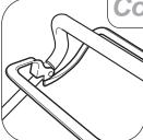
Operate all control levers several times and ensure that the cables move freely. Check that the cutterblade stop and ground drive clutch levers return freely to their rest position when released.
