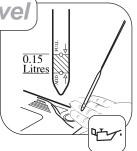
The oil level is correct when it is at the **full** mark on the dipstick. **DO NOT OVERFILL.**
