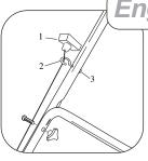
Operate the engine stop lever towards the handlebar and very slowly pull the engine start grip (1) away from the engine until there is sufficient slack in the rope to enable it to be threaded into the rope guide (2). Release the start-grip until it rests against the rope guide as shown. Finally tighten the nut (3) to secure the rope guide.
