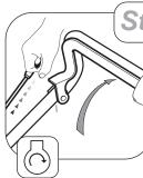
Stand behind the mower and hold the handlebar together with the engine stop lever with your left hand. With your right hand hold the engine start - grip and pull slowly until resistance is felt, then pull rapidly to crank the engine. Carefully return the start grip to the storage position when the engine starts.
