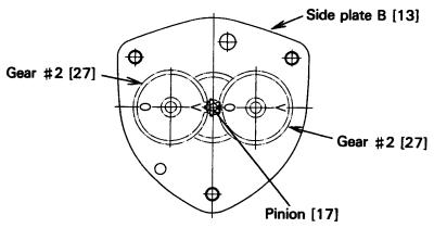
Figure 6-4 Gear Train Assembly
