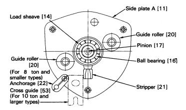
Figure 6-3 Side Plate Assembly
