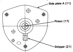
Figure 6-2 Side Plate / Load Sheave Assembly
