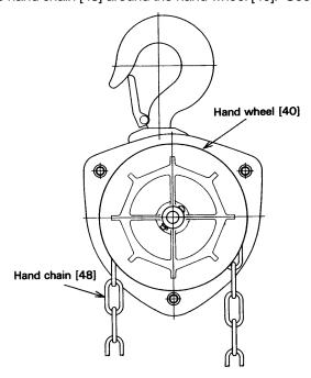
Figure 6-10 Hand Wheel Assembly
