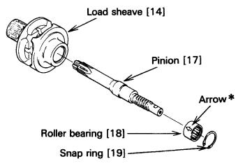
Figure 6-1 Load Sheave/Pinion Assembly
