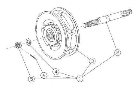
Figure 9-4 Slip Clutch
