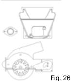
Latch "closed "with blower cover in place. Burn pot clean-out is closed.
