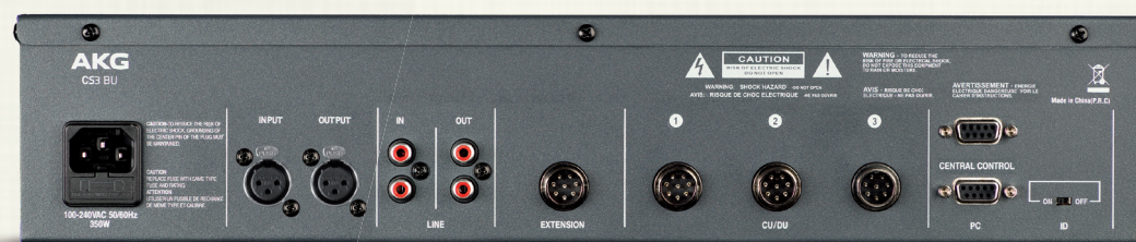
CS3 BASE UNIT | CONNECTIONS
