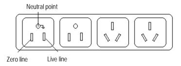
Figure 3-6 Recommended AC power socket
