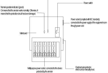
Figure 4-1 Diagram of lightning arrester
