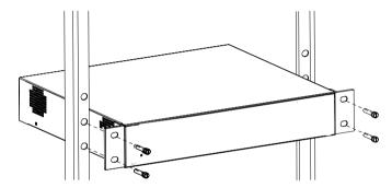
Figure 3-1 Mounting the switch into a 19-inch cabinet
