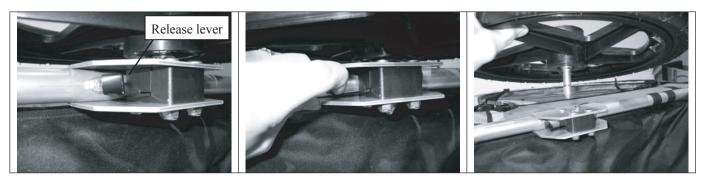
The release levers are located between the wheel bracket plates below the frame near the rear of the trailer. There is one lever on each bracket. They can be accessed from the rear.
