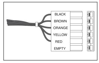
Figure 6-4. – Six Pin Connector Wire Colors
