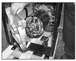
Figure 7-7. – Remove Bearing Carrier
