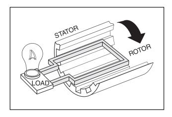
Figure 1-3. – A Simple Revolving Field Generator
