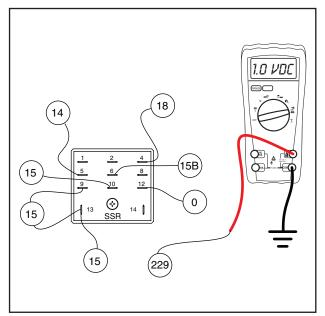
Figure 6-47. – Testing Wire 229 to Ground
