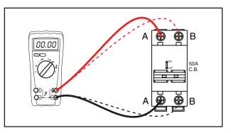
Figure 6-7. – 50 Amp Breaker Test Points
