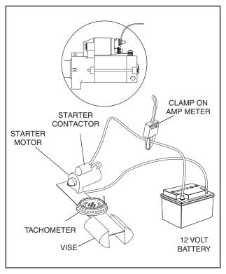
Figure 6-34 – Testing Starter Motor Performance
