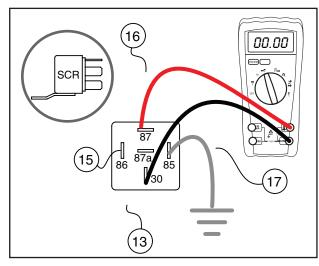
Figure 6-35. - Starter Contactor Relay Test
