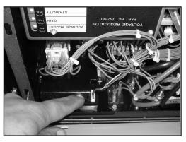
Figure 7-2. – Stepper Motor Harness
