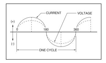
Figure 1-5. – Alternating Current Sine Wave
