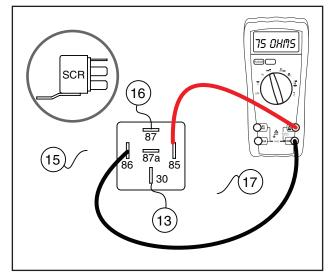
Figure 6-55. – Testing Starter Contactor Relay (SCR)
