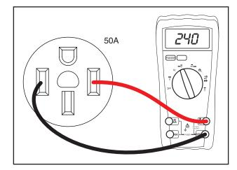
Figure 6-1. – VOM Test Leads Connected to 50A Outlet
