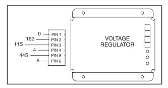
Figure 6-11. - Voltage Regulator Pin Connector Wire Number Locations
