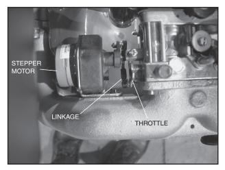
Figure 6-2. – Stepper Motor, Linkage and Throttle Seen From Above
