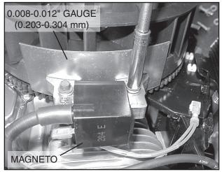
Figure 6-49. – Setting Ignition Magneto (Armature) Air Gap
