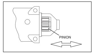
Figure 6-30. – Check Pinion Gear Operation
