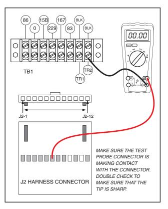
Figure 6-62. – Check TR2 Wiring
