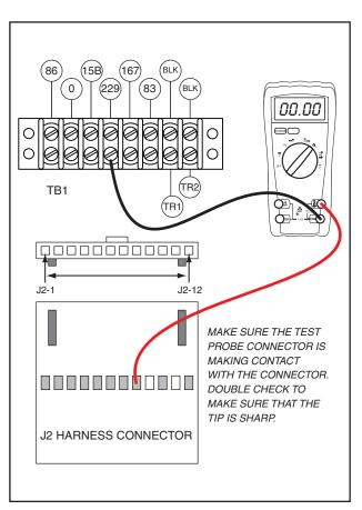
Figure 6-48. – Testing Wire 229 Between J2 Connector and Terminal Block 1 (TB1)
