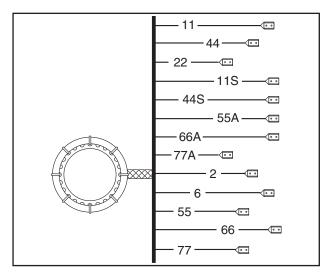
Figure 3-9. – Stator Winding Leads
