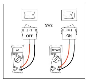
Figure 6-59. – Check Idle Control Switch (SW2)
