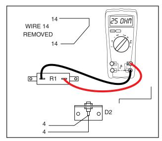
Figure 6-17. – Diode Test Step 9
