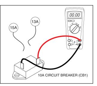
Figure 6-26. – Testing 10 Amp Breaker
