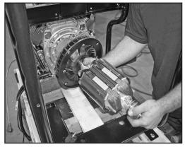
Figure 7-9. – Remove Rotor
