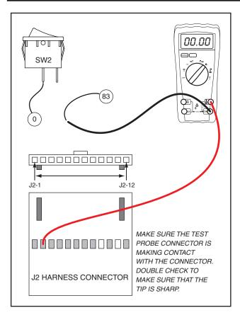
Figure 6-60. – Check Idle Control Wiring
