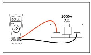
Figure 6-8. – 20/30 Amp Breaker Test Points
