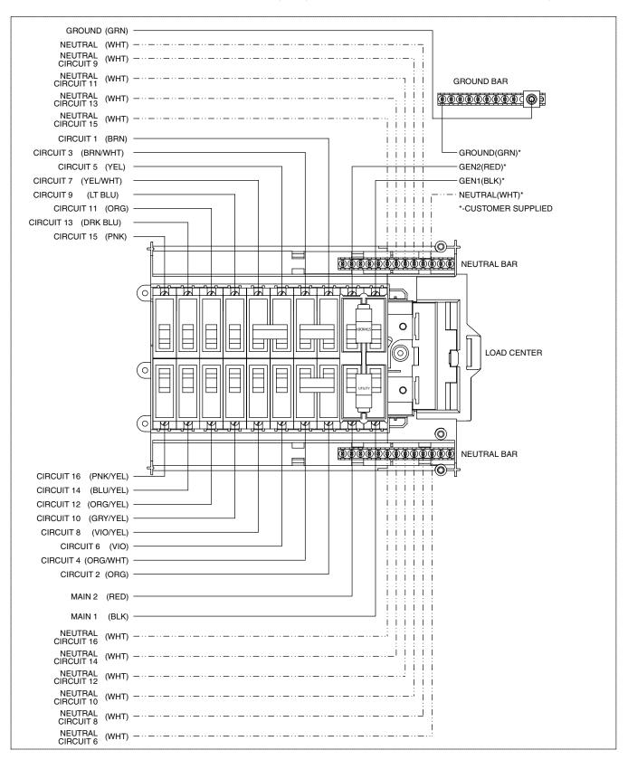
Wiring Diagram, 17.5 kW Manual Transfer Switch – Drawing No. 0G1065
