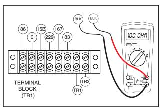
Figure 6-61. Check Idle Transformer Wiring
