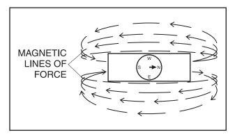
Figure 1-1. – Magnetic Lines of Force
