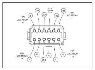
Figure 6-18. - C1 Connector, Female Side
