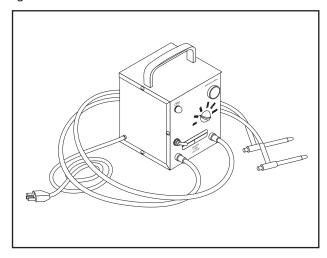
Figure 3-8. – One Type of Hi-Pot Tester
