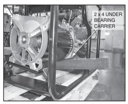
Figure 7-6. – Support Alternator
