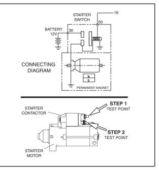
Figure 6-28. – The Starter Contactor (SC)
