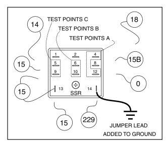
Figure 6-43. - Start Stop Relay (SSR) Energized
