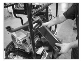
Figure 7-5. – Remove Muffler
