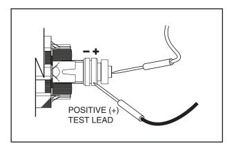
Figure 3-10. – Testing Rotor Insulation
