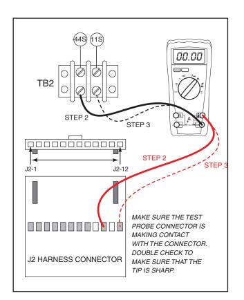
Figure 6-58. – Check Wires 11S & 44S
