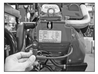
Figure 6-37. – Testing Ignition System
