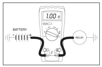
Figure 2-4. – A VOM as an In-line meter
