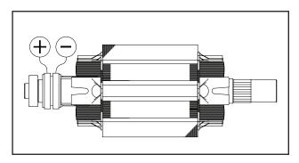
Figure 3-2. – The 2-Pole Rotor Assembly
