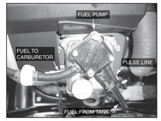
Figure 6-50. – Fuel Pump and Fuel Lines
