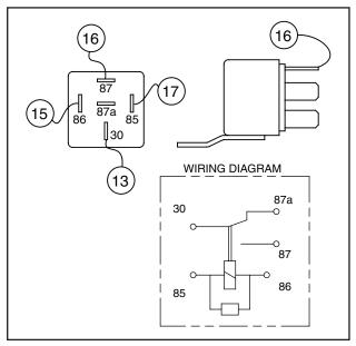
Figure 6-13. – Starter Contactor Relay
