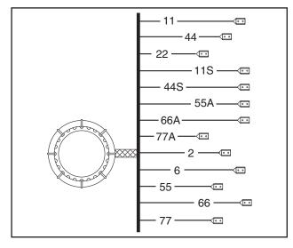
Figure 3-3. – Stator Assembly Leads
