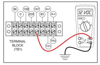
Figure 6-45. – Test Wire 167, Step 3
