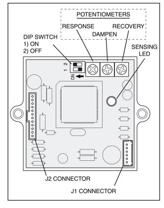
Figure 4-1. – Printed Circuit Board
