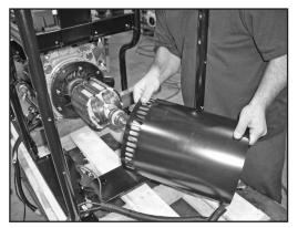
Figure 7-8. – Remove Stator
