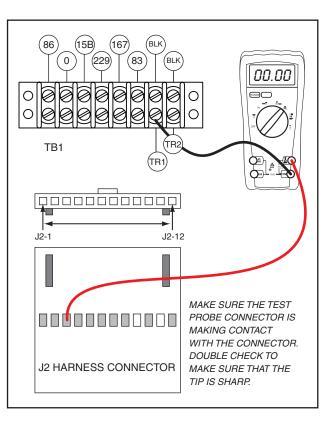
Figure 6-63. – Check TR1 Wiring
