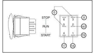
Figure 6-36. – Start-Run-Stop Switch (SW1)
