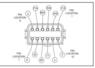
Figure 3-10. – C1 Connector Pin Location Numbers (Female Side, Located to the Right When Facing the Control Panel)
