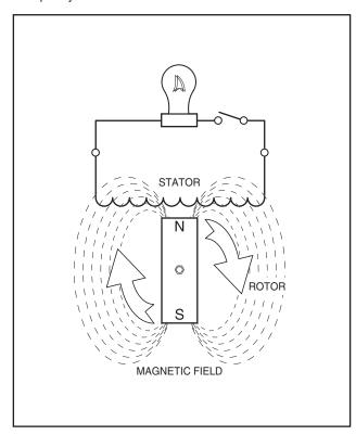
Figure 1-4. – A Simple AC Generator
