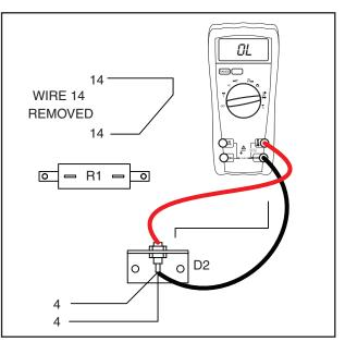
Figure 6-15. – Diode Test Step 5
