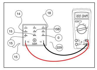
Figure 6-54. – Testing Start Stop Relay (SSR)
