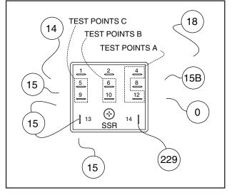
Figure 6-42. – Start Stop Relay (SSR) Not Energized
