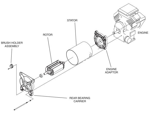
Figure 3-1. – AC Generator Exploded View
