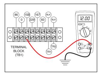
Figure 6-5. – Testing Wire 15B
