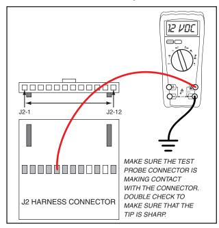
Figure 6-44. – Test Wire 167, Step 2
