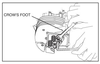
Figure 6-52 – Tightening the Jam Nut
