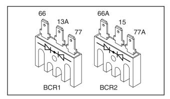
Figure 6-25. – Battery Charge Rectifier
