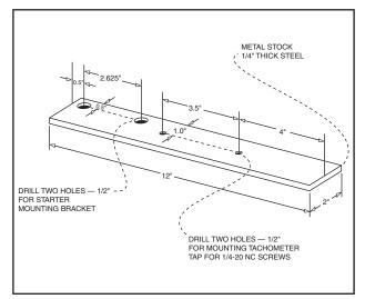
Figure 6-33. – Test Bracket Dimensions
