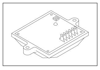
Figure 3-7. – Typical Voltage Regulator Found on 17.5 Units
