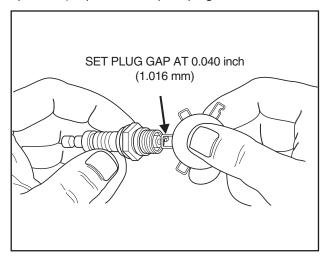
Figure 6-39. – Setting Spark Plug Gap
