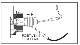
Figure 6-22. – Testing at Slip Rings
