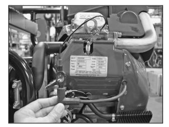
Figure 6-38. – Checking Engine Miss
