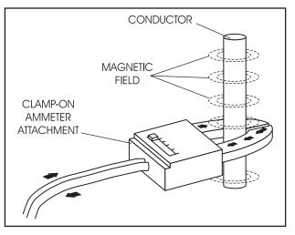
Figure 6-31. – Clamp-On Ammeter
