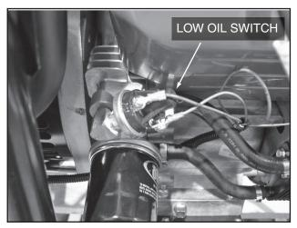
Figure 6-53. – Low Oil Pressure Switch
