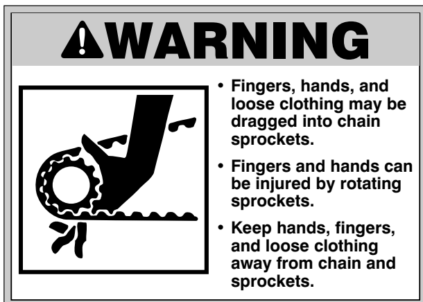
warning label located (inside housing) next to sprockets on back of operator
