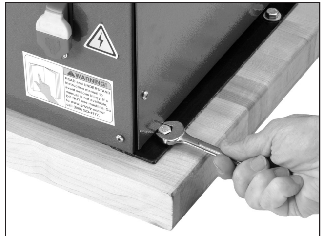
Figure 5. Installing sander onto bench top.
