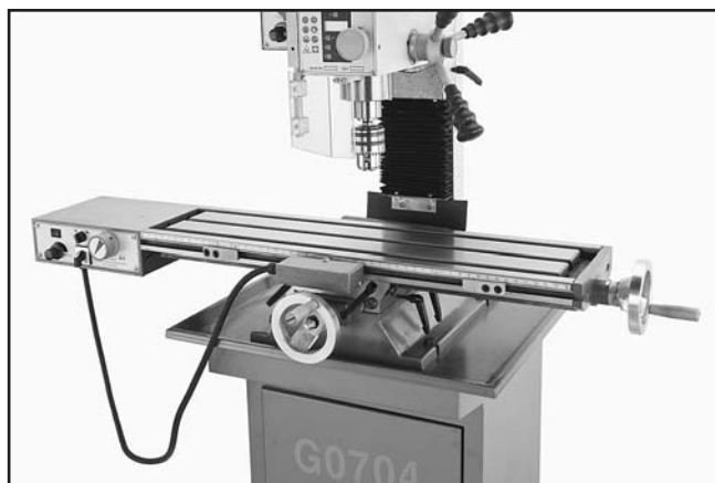
Figure 19. Power feed installation complete.
