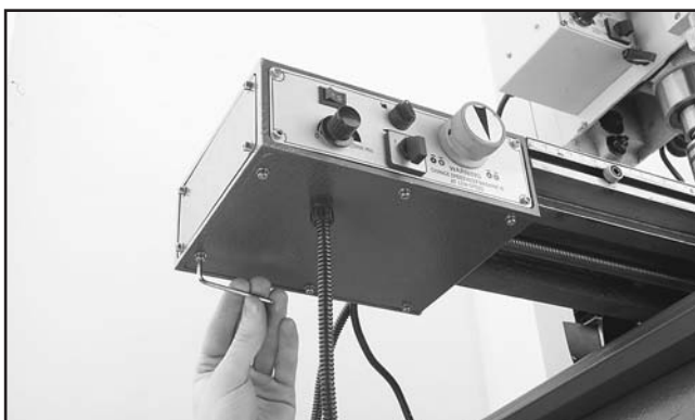
Figure 8. Replacing bottom cover.
