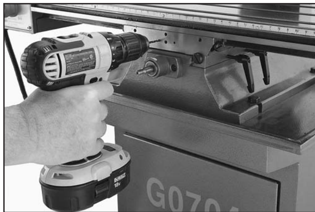
Figure 14. Drilling holes for limit switch assembly.
