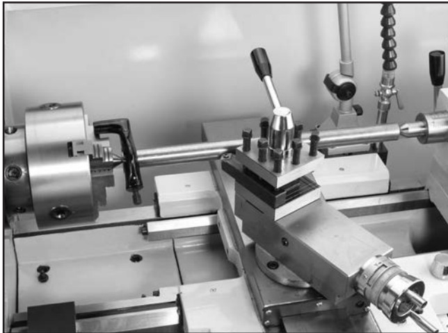
Figure 33. Example of stock mounted between the centers.
