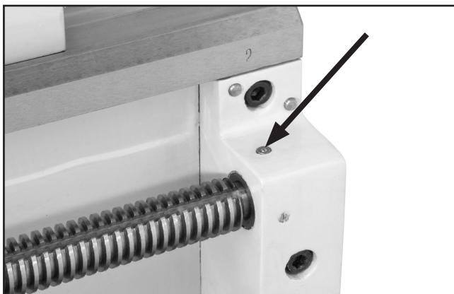
Figure 52. Lead screw end cap bushing.
