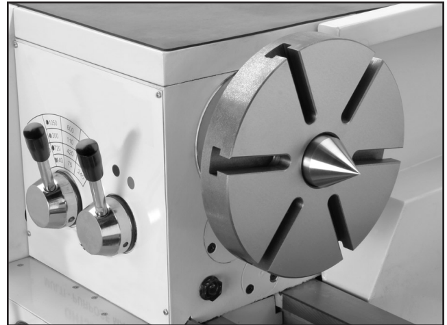
Figure 25. Faceplate and dead center setup.
