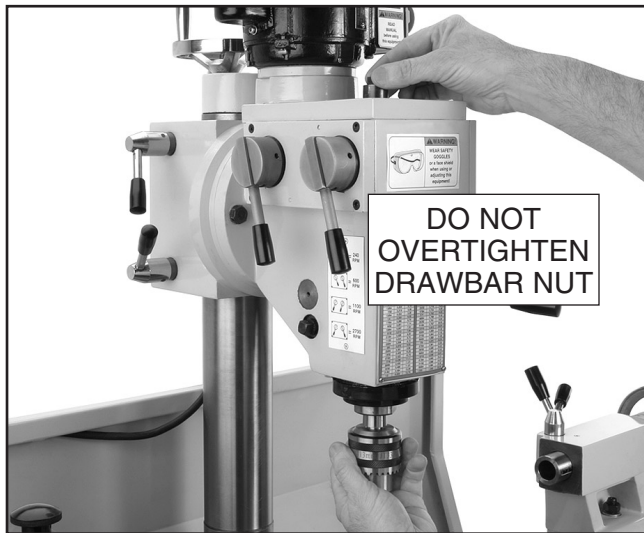
Figure 44. Aligning drawbar with chuck arbor.
