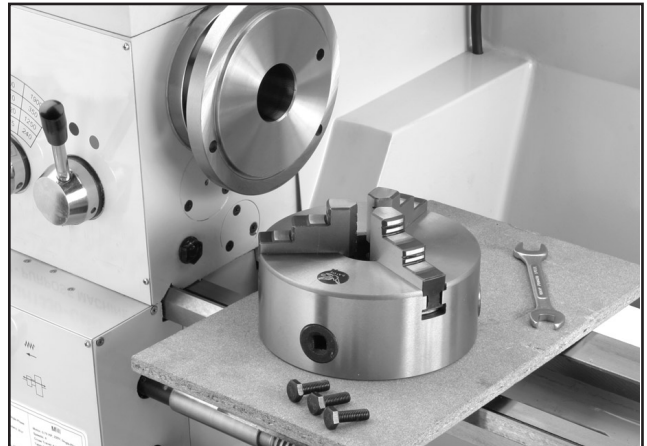
Figure 10. Chuck mounting components.
