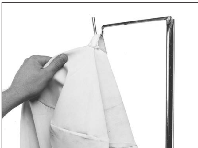
Figure 22. Attaching upper filter bag.
