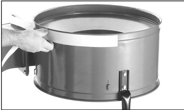
Figure 17. Installing wide foam strip.
