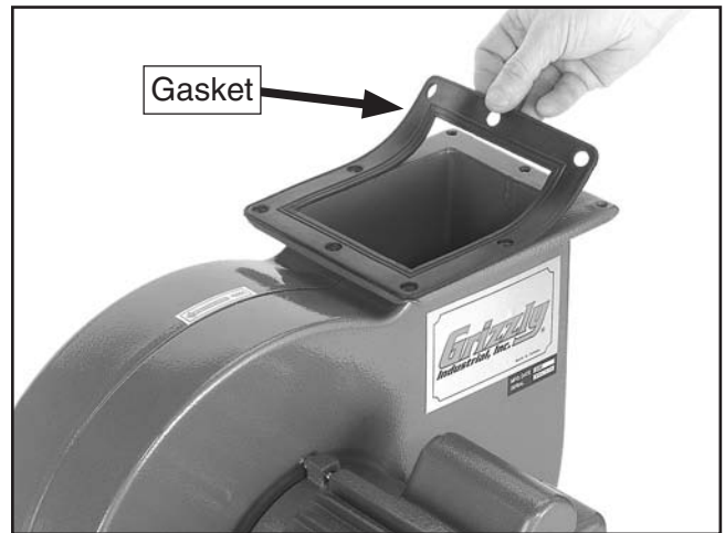
Figure 11. Positioning impeller outlet gasket.
