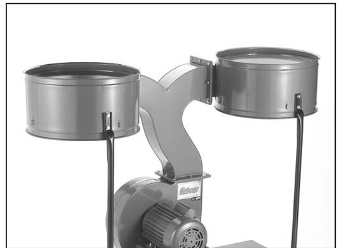
Figure 16. Collectors installed (G0562Z shown).
