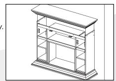
Locate the left speaker frame. Position the frame inside the opening beneath the top of the mantel. From the back, line up the holes, insert and tighten the 2 wing nut and lock washers.
