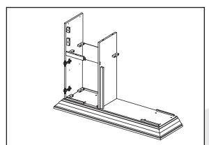
Locate the left top shelf. Position it on the 4 supports on the left side panels – 2 on the exterior and 2 on the interior panels. From below line up the holes in the supports with those of the top shelf, insert and tighten the 4 wing nuts and lock washers.
