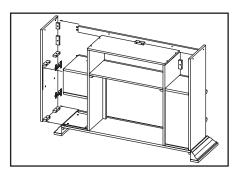
Line up the 2 holes between the right exterior side panel and the base, insert and tighten the 2 wing nuts and lock washers. Line up the holes between the 2 supports on the right exterior side panel and the holes on the right top shelf. From below insert and tighten the 2 wing nuts and lock washers.
