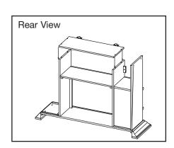
Locate the support panel for the top of the mantel. Insert the dowels on the side of the support panel into the dowels holes in the left side panel (exterior). Line up the support in the middle of the support panel with the hole in the central top shelf. From the top, insert and tighten the 1 wing nut and lock washer.
