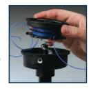
9. When operating for the first time after changing the spool of line ensure to test the assembly by running the line trimmer in a safe location. The line may not be fully extended so you may need to "bump" the head at full speed to feed the line to the correct length.
