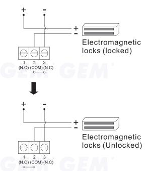
No need to power in. It has a switch for motoring in case of emergency when glass is broken; the contacts change from N/C to N/O.
