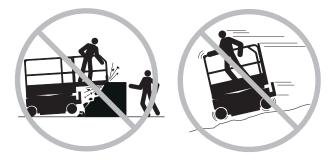
Limit travel speed according to the condition of the ground surface, congestion, slope, location of personnel and any other factors which may cause collision.
