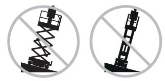
Models with outriggers: Do not lower the outriggers unless the machine is on a firm surface. Avoid drop-offs, holes, unstable or slippery surfaces and other possible hazardous conditions.
