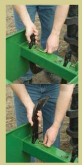
**Choose from three** scarifier depth adjustments to meet a variety of ground conditions. Adjustments are easy! Simply remove the steel pin, and raise or lower the scarifier to increase or decrease ground penetration. Scarifier shanks can be stored on the scarifier beam when using the box blade for other tasks.
