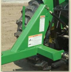
A heavy, welded mast and 4x4-inch tubular steel frame deliver added strength and rigidity.
