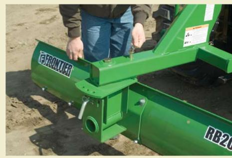
Adjusting the angle is easy. Simply remove the steel pin and rotate the blade to the desired setting, or swing it around for backfilling.
