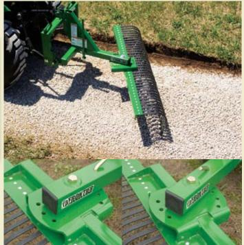
Achieve the desired raking profile by adjusting the time beam in one of five different positions forward and three positions in reverse. Simply remove the steel pin and rotate the beam to the desired setting.
