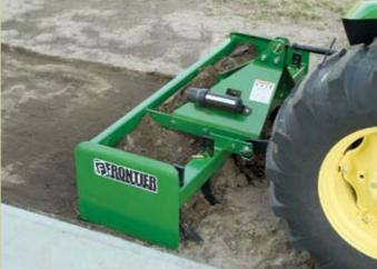
Heavy-duty, concave back plate with formed upper edge provides added rigidity and strength for trouble-free performance.
