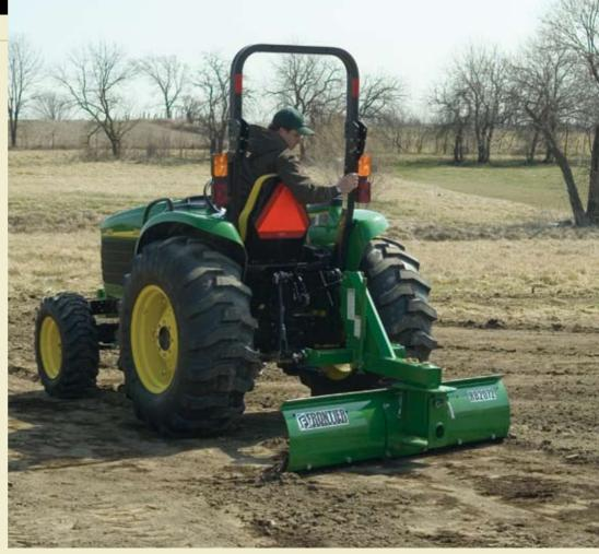
A formed, upper moldboard edge increases rigidity. Moldboard thickness is 3/16-inch for RB2060 and 1/4-inch for RB2072 and RB2084.
