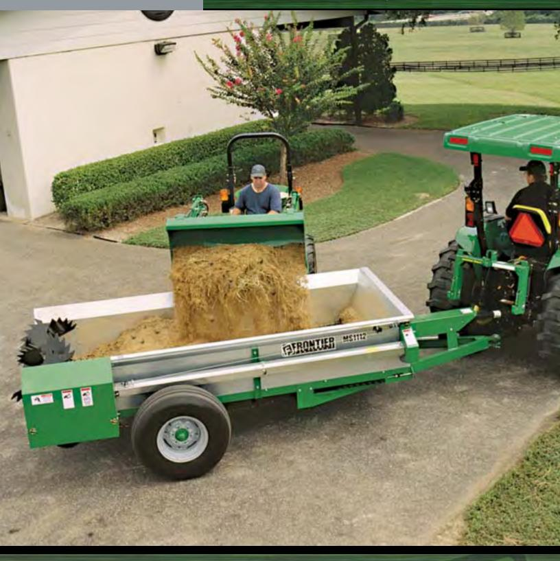
25- to 175-bushel capacity • Ground- and PTO-driven models
