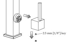
6. Find the small notch at the base of the chrome ring cap and carefully pry up against this to remove the cap.
