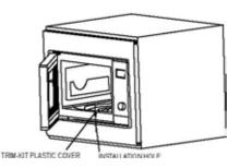
2 Open the door; fix the oven to the cabinet with SCREW at the INSTALLATION HOLE of TRIM KIT. Then fix the TRIM-KIT PLASTIC COVER to the INSTALLATION HOLE.
