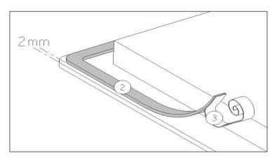
Stick the gasket (2) two millimeters from the external edge of the glass, after removing the protection sheet (3).
