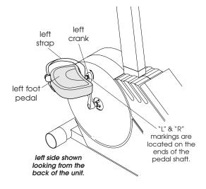
**Figure 7** - Install Foot Pedals
