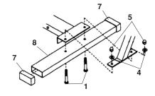
M8 x 60mm CARRIAGE BOLT (1) M8 WASHER (4) M8 ACORN NUT (5) END CAP (7) REAR FOOT TUBE (8)
