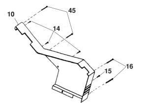
RIGHT REAR COVER (10) M4 X 12mm PHILLIPS SCREW (14) M4 x 16mm PHILLIPS SCREW (15) M5 x 115mm PHILLIPS SCREW (16) M5 x 50mm PHILLIPS SCREW (45)
