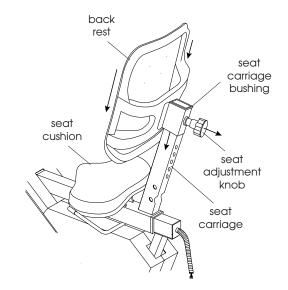
Figure 4c - Install Back Rest
