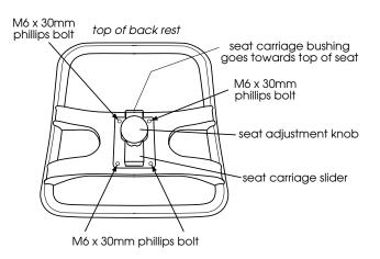
Figure 4b - Install Seat Carriage Slider
