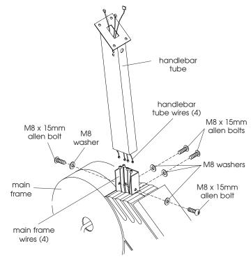
Figure 6 - Install Handlebar Tube
