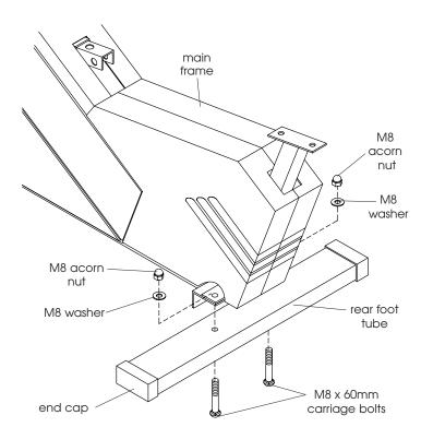
Figure 2 - Install Rear Foot Tube
