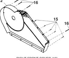
RIGHT FRONT COVER (12) M4 x 16mm PHILLIPS SCREW (15) M5 x 115mm PHILLIPS SCREW (16)
