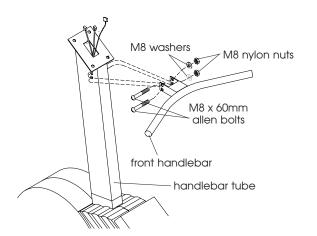
Figure 8 - Install Front Handlebar
