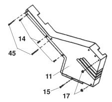
LEFT REAR COVER (11) M4 X 12mm PHILLIPS SCREW (14) M4 x 16mm PHILLIPS SCREW (15) M5 NUT (17) M5 x 50mm PHILLIPS SCREW (45)
