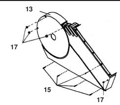
LEFT FRONT COVER (13) M4 x 16mm PHILLIPS SCREW (15) M5 NUT (17)
