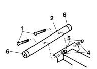
M8 X 60mm CARRIAGE BOLT (1) FRONT FOOT TUBE (2) M8 WASHER (4) M8 ACORN NUT (5) ROLLER (6) 28
