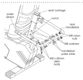
Figure 5 - Install Rear Handlebar
