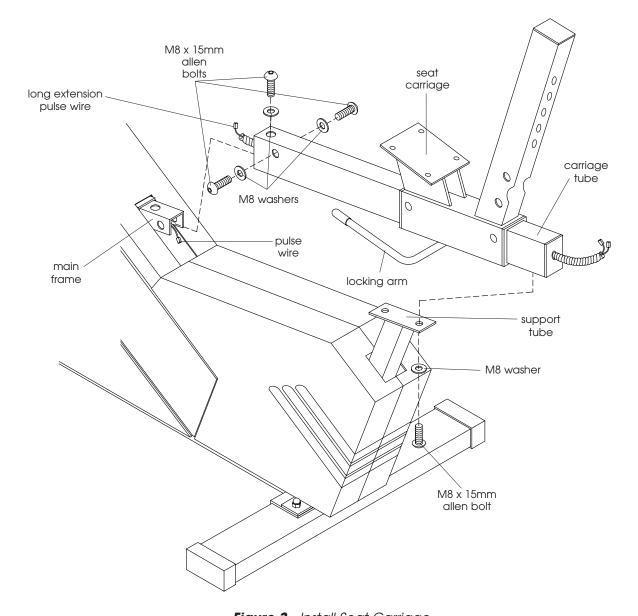
Figure 3 - Install Seat Carriage
