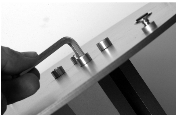
Fix the two stands to the plate, using the screws and the Allen key
