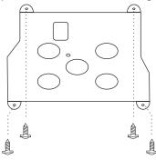
3. Match the position of installation bracket and installation plate with screw A.
