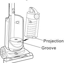
Push the dust compartment into the main body as shown to reattach.
