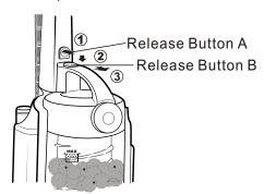
Turn the spinner handle several times in the direction shown to empty the dust compartment.
