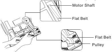
Place the agitator assembly into the grooves in the nozzle head, making sure that the new flat belt slides securely into the guide.
