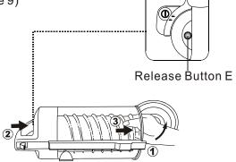
Clean the main filter and prefilter with a soft-bristled brush and rinse with cold water. Allow both items to dry completely.
