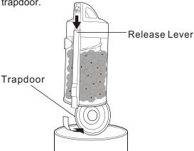
Press the release button A meanwhile press the release button B to remove the dust compartment.
