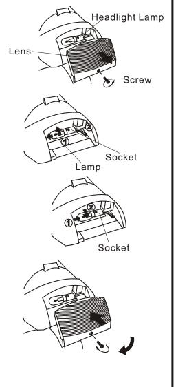
Reattach the lens and fasten the screws.
