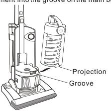
Push the dust compartment into the main body as shown to reattach.
