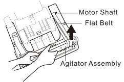
Place a new flat belt onto the motor shaft and pulley.
