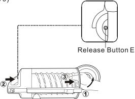
Clean the main filter and prefilter with a soft-bristled brush (not included) and rinse with cold water. Allow both items to dry completely for 24 hours.
