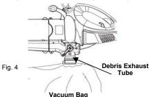
4. To remove the vacuum bag, loosen the velcro strap and pull the vacuum bag off of the debris exhaust tube. (Fig. 5)
