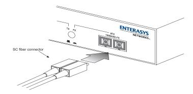
Figure 2-5. Inserting an SC Fiber Connector into the Fiber Port
