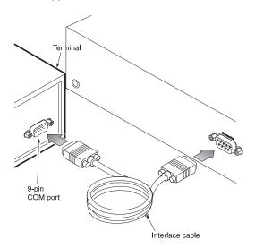
Figure 2-2. Connecting a Terminal to the Console Port
