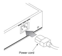
Figure 2-3. Connecting the Power Cord
