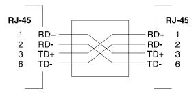
Figure A-1. External Crossover Cable Wiring
