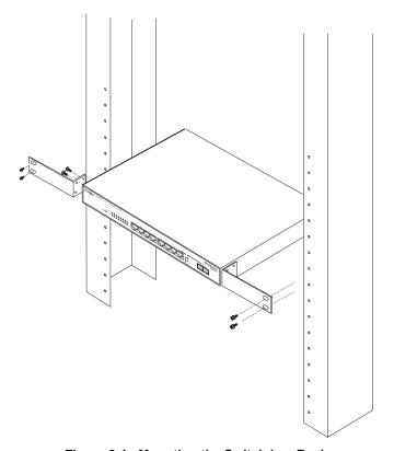
Figure 2-1. Mounting the Switch in a Rack
