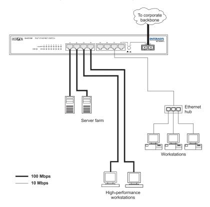
Figure 1-3. Client/Server Network Application
