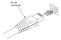
Figure 2-4. Inserting an RJ-45 Connector into a Port
