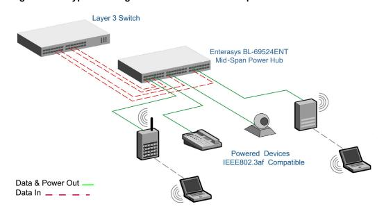
Figure 2-2 Typical Configuration for a 24-Port Mid-Span Power Hub
