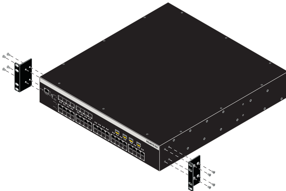
Figure 3-1 Attaching Rack-mount Ears to Enterasys Matrix N SA 2G4072-52
